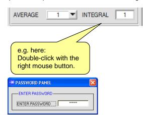
Offset calibration can be accessed by double-clicking with the right mouse button exactly at the frame below **INTEGRAL** in the **PARA** tab.
