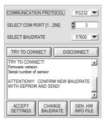
When the new baudrate information has been successfully sent, the sensor operates with the new baudrate. A window will pop up, prompting you to select **EEPROM** and then to press **SEND**. After a hardware reset the new baudrate only will be used when **EEPROM** and **SEND** have been pressed.
