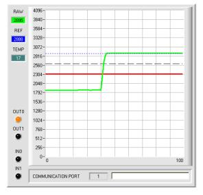
When the current measurement value **RAW** (green line) rises above the hysteresis threshold (black line) again, the output **OUT0** also changes to +24V again (signal is OK). This is visualised by the **OUT0** LED.
