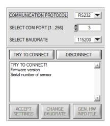
The baudrate for data transfer through the RS232 interface can be set by means of the **SELECT BAUDRATE** drop down menu and **CHANGE BAUDRATE** function field.
