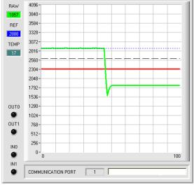
When the current measurement value **RAW** (green line) falls below the switching threshold (red line), the output **OUT0** changes to 0V (error). This is visualised by the **OUT0** LED.
