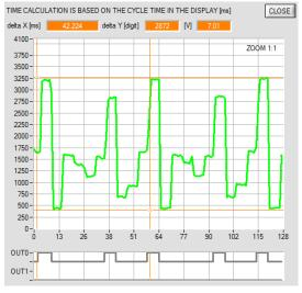
The zoom function in the graph can be activated by holding the control key (CTRL) and drawing a window with the mouse. A click on **ZOOM 1:1** cancels the zoom function again.
